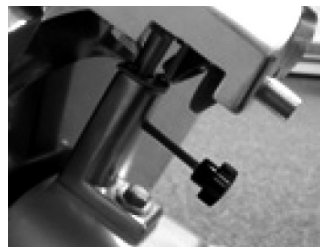
3. Secure the sharpening device to the machine by tightening the holder. Check to make sure that the sharpening device is well secured before using the machine.
