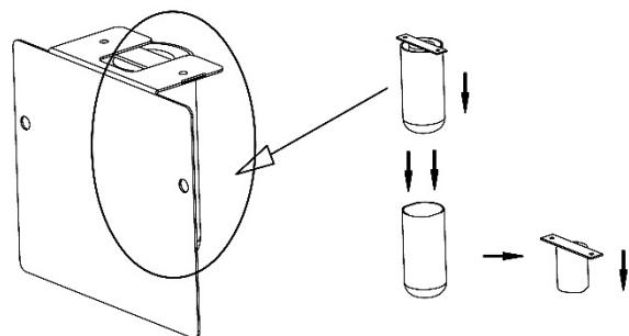
Pull the cover of the UV lamp downwards and replace the lamp.
