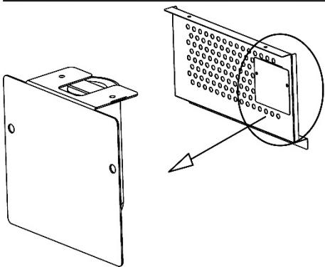
Remove the cover. The UV lamp is attached to this.
