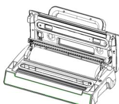
Make sure the bag cutter is on one end of the cutter rack, then put the cutter rack to the back
