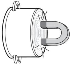
Ensure that the pot bears an inscription stating its suitability for cooking with induction current, or perform the following magnet test:
